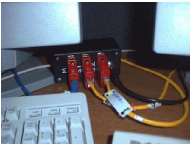
Figure 2. A fabricated box that handles genlocking and data locking through parallel port connections.
